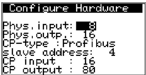
The cam controller has a total of 16 + 80 = 96 outputs and 8 + 16 = 24 inputs. The outputs 17 - 80 and the inputs 9 - 24 are simulated by the CamCon CP16, that is connected to the CamCon DC16 via the external interface.
