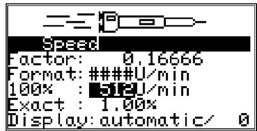
**Example:** With a 100% value of 512 rot/min you need to divide through 64, which corresponds to a shifting operation of SRW 6.
