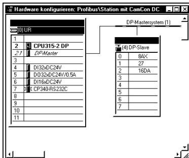
To the left you see an example for a CPU315-2 DP and a CamCon CP16/P/IO. The CP16 has a communication - module (8AX), an input - module (27) with 96 inputs and an output - module (16DA) with 16 outputs.
