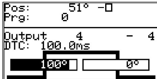
If you now press the **←** key or the **→** key, all the cams of this output are shifted by one increment. In this case the cams are directly taken over into the memory without the use of the **CR** key (unlike before). The shifting process is ended by pressing either the **CR** key or the **ESC** key.
