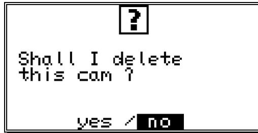
To delete the cam, move the cursor to "yes" with the
