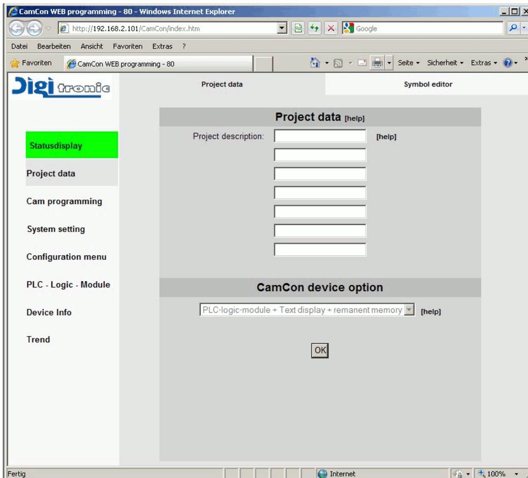
Now you can configure the CamCon DC190 completely on this WEB - page as it is written in the manual or you can fully configure the DC190 by the ControlLogix CPU PLC via the DC190 Program TAGs.
