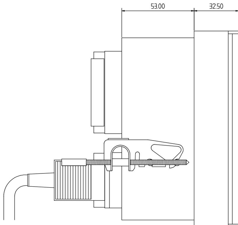
Fig.: Drawing to aid the installation of CamCon
