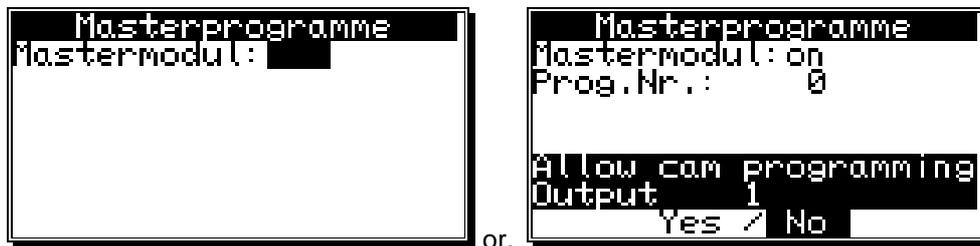
Here you are able to define Cams for different products and programs. They could be necessary if your plant produces different types of products that have only very little differences concerning their Cam-adjustment. You are able to save a lot of storage for Cams (EE-Prom), because these mastercams do not need to be programmed multiple.
