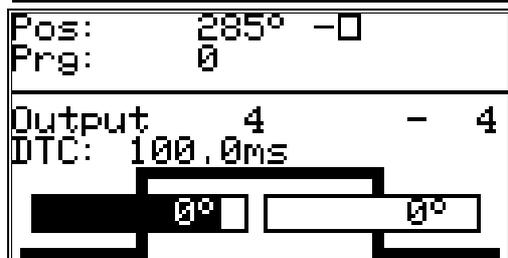
4. Press the **INS** key to enter the cam activation point for an additional cam. The cursor moves to the input field for the cam activation point; a stylized cam starts to blink simultaneously.
