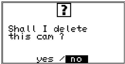
To delete the cam, move the cursor to "yes" with the
