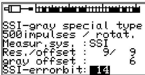
**Attention:** *The position of the data bits can be seen in the graphic in the upper part of the display. You can determine the positions of the LSB, HSB and errorbits quite easily by moving the measuring system.*
