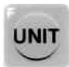
By pressing this key, you can initiate the following functions in a multi axis system: input of unit (axis) numbers, change the 7-segment display from "Speed" and "Prg" to "Position" and adjust the contrast setting of the LCD.
