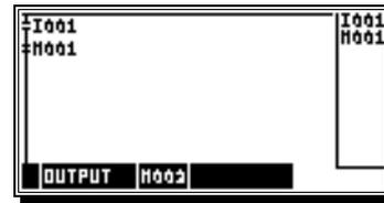
Register 2 is activated for one cycle, when the signal on input 1 changes from 0 to 1.
