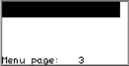
By pressing the keys **▼** and **▲** you now select the lines that you wish to edit and confirm this with the **CR** key. If lines 1, 2 or 7 are selected, the line can either be defined as "1 text" or "2 variables" lines and can thus be used as a heading.
