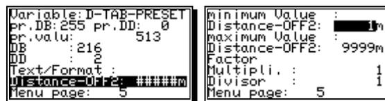
The "D-TAB-Preset" variables is used for simply feeding in parameters off an PLC-Logic-Module and needs 10 parameters itself:
