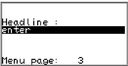
By pressing the **CR** key the "heading" is saved and the program returns to the line selection menu. Here you can again select the next line with the **▼** and **▲** keys and by entering **CR**, you either enter the "2<sup>nd</sup> heading" or the first variables.
