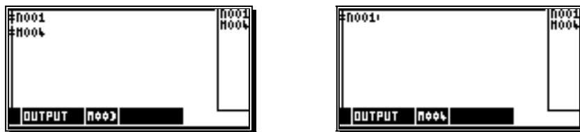
If the cam N001 is switched off (negative edge), the M005 flag is reset.
