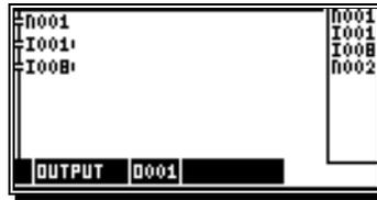
Output 1 of the CamCon is enabled when inputs 1 and 8 are active.
