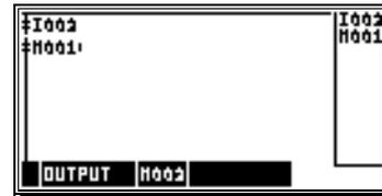
Register 2 is activated for one cycle, when the signal on input 2 changes from 1 to 0.
