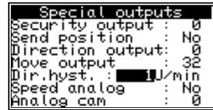
Via the move detection output, the controll module detects a stop of the machine to be able to display the last controlled curve correctly.
