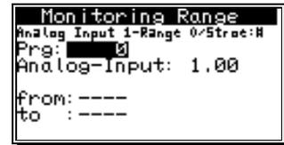
**from:** Starting point of a monitoring range in units of actual value, e.g. degree.
