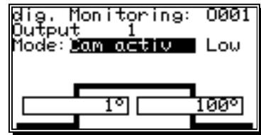
If a signal input within the window Cam gets inactive a message is displayed, respectively the corresponding PLC - output switches to "1" (e.g. M001 or O001).
