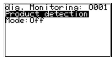
After having pressed the key **[CR]** the text is saved and the device switches on to the selection of a controlling mode. Six different modes and one automatic detection mode may be adjusted here. These modes are: **"Off"**, **"Static"**, **"Range"**, **"Counter min."**, **"Counter exact"**, **"Cam active"** and **"Auto"**.
