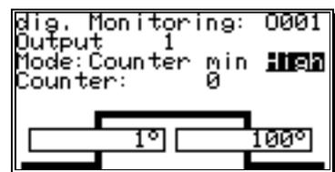
If a signal input gets active out of a window Cam or if not enough negative edges (at least three) are counted, a message is displayed respectively the corresponding PLC - output is set to "1" (e.g. M001 or O001). If more than three edges are detected, no error is displayed.
