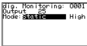
By pressing the keys **[CR]** the particular controlling is adjusted in relation to the production ssettings. After having entered the user key (for Cam programming) a free text with a maximum length of 17 characters is entered wich describes the controlling's function.
