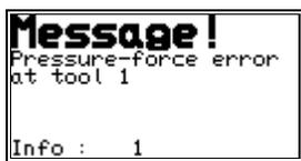
By the error - report system integrated into the PLC-Logic-Module it is possible to report an error message to the operator of the plant.
