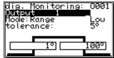
A message is displayed respectively the corresponding PLC output is set to "1" (e.g. M001) if the input signal in the inner tolerance range is active and active above the outer tolerance range. Both tolerance ranges are calculated from an entered Cam.
