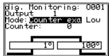
If the signal input out of the window cam is active, or more than n (e.g. 3) negative edges are counted a message is displayed respectively the corresponding PLC-output is set to "1" (e.g. M001 or O001).
