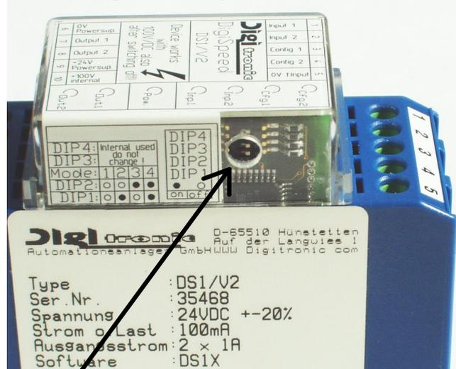
To adjust the dip-switch use a small screwdriver or an bent paper clip.
