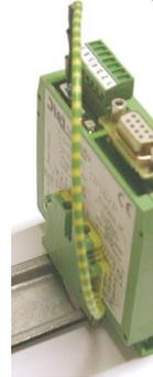
**Note:** The analog - digital - converter has to be switched to the end of the interface row.
